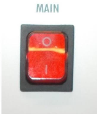
Figure 7: Main switch 230V
